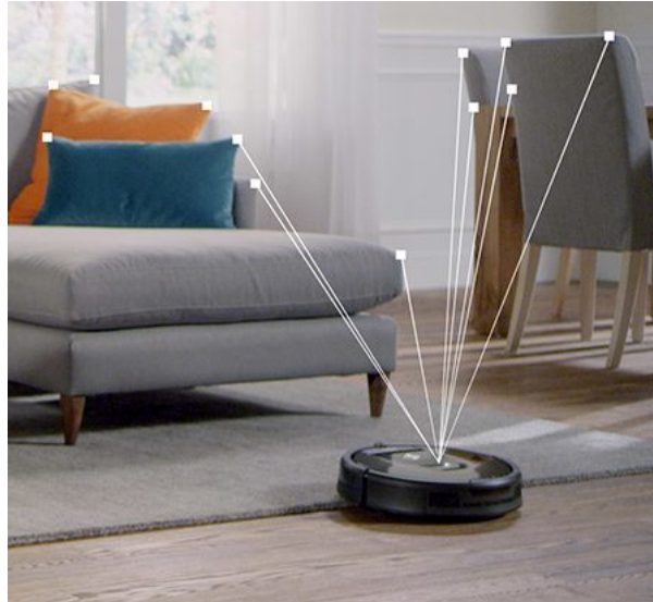
Figure 1.3: SLAM system of Roomba robots based on visual features, by iRobot.
