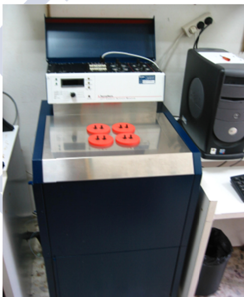
Figure 2.7. Microcalorimeter 2277 Thermal Activity Monitor (TAM) Thermometric AB.
