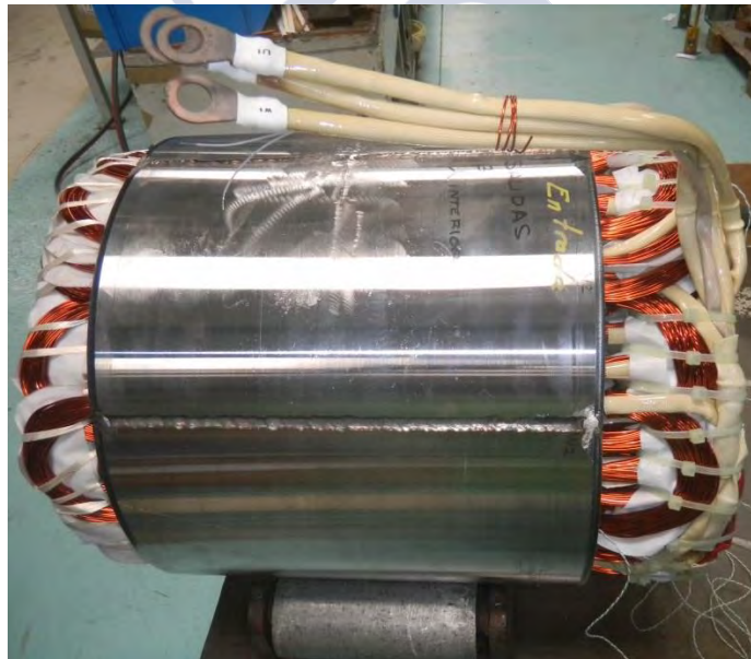
Figure 3.21. IkerMAQ stator, the end-windings at both sides are clearly visible.
