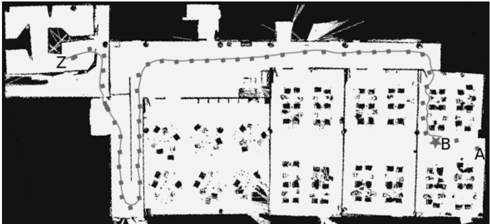
(b) High localization performance example when using all the sensors in our robot (laser, wifi and compass).
