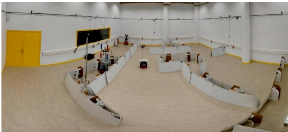
Figure 5.2: 100m^2 robotics laboratory where we have conducted several route reproduction tests. We set up an environment with 5 rooms, and recorded and reproduced several routes while two humans were walking around.
