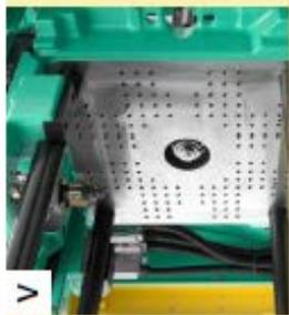
V position: vertical arrangement of the second injection unit above the mould.
