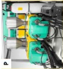
P position: second injection unit horizontal and parallel to the first.
