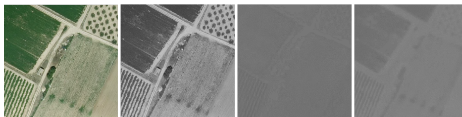
Figure 1.: From left to right: RGB image, \mathbf{Y} (luminance), \mathbf{C}_b (blue-difference) and \mathbf{C}_r (red-difference) channels.
