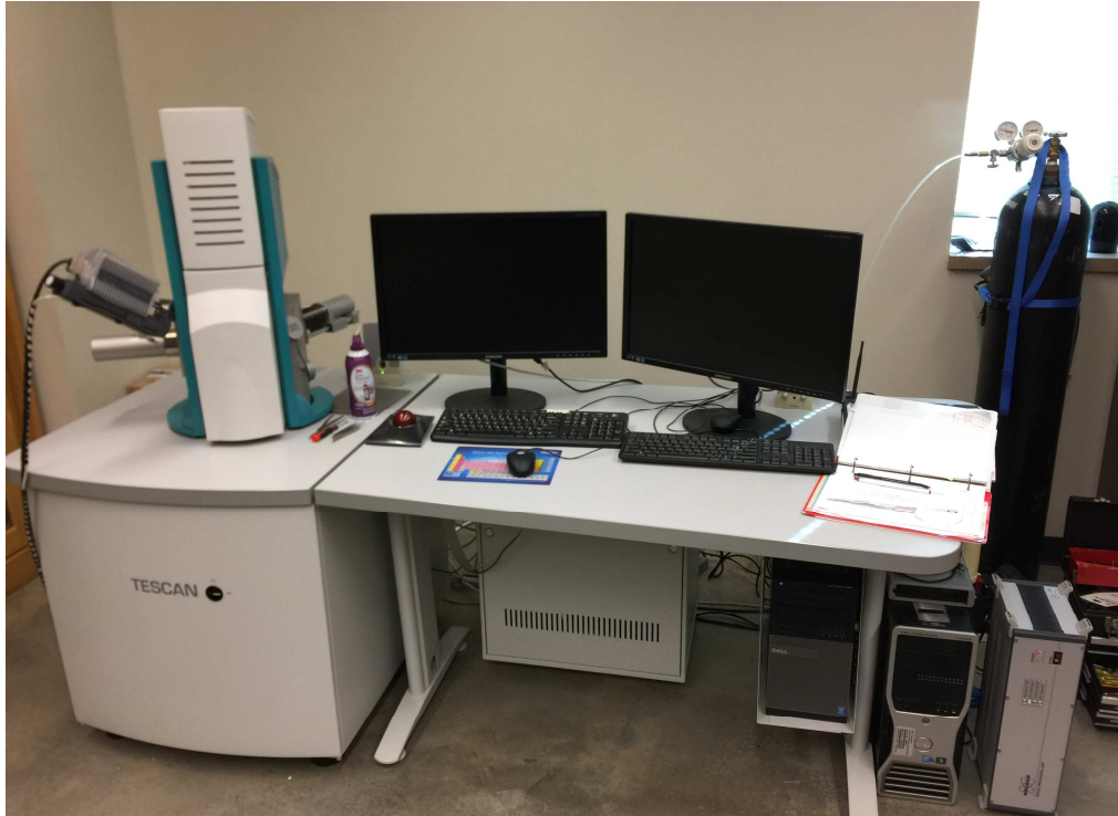
Figure 7. TESCAN VEGA 3LMU scanning electron microscopy in Department of Geosciences at UMKC.
