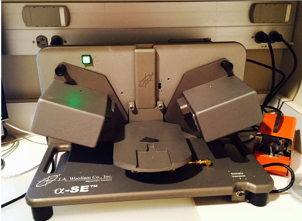
Figure 10. The ellipsometry system alpha-SE from J. A. Woollam Co in UMKC Department of Physics and Astronomy.
