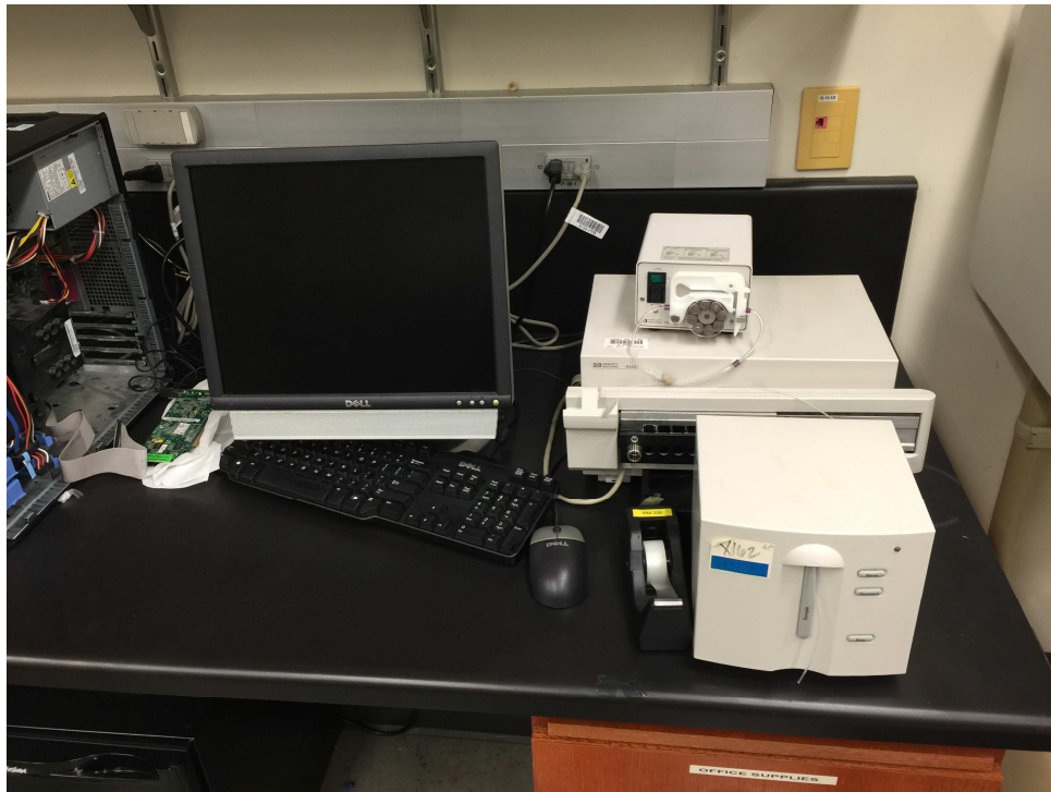
Figure 11. An ultraviolet-visible spectroscope Agilent/HP 8453 UV-Visible Spectrophotometer in the department of physics, UMKC.
