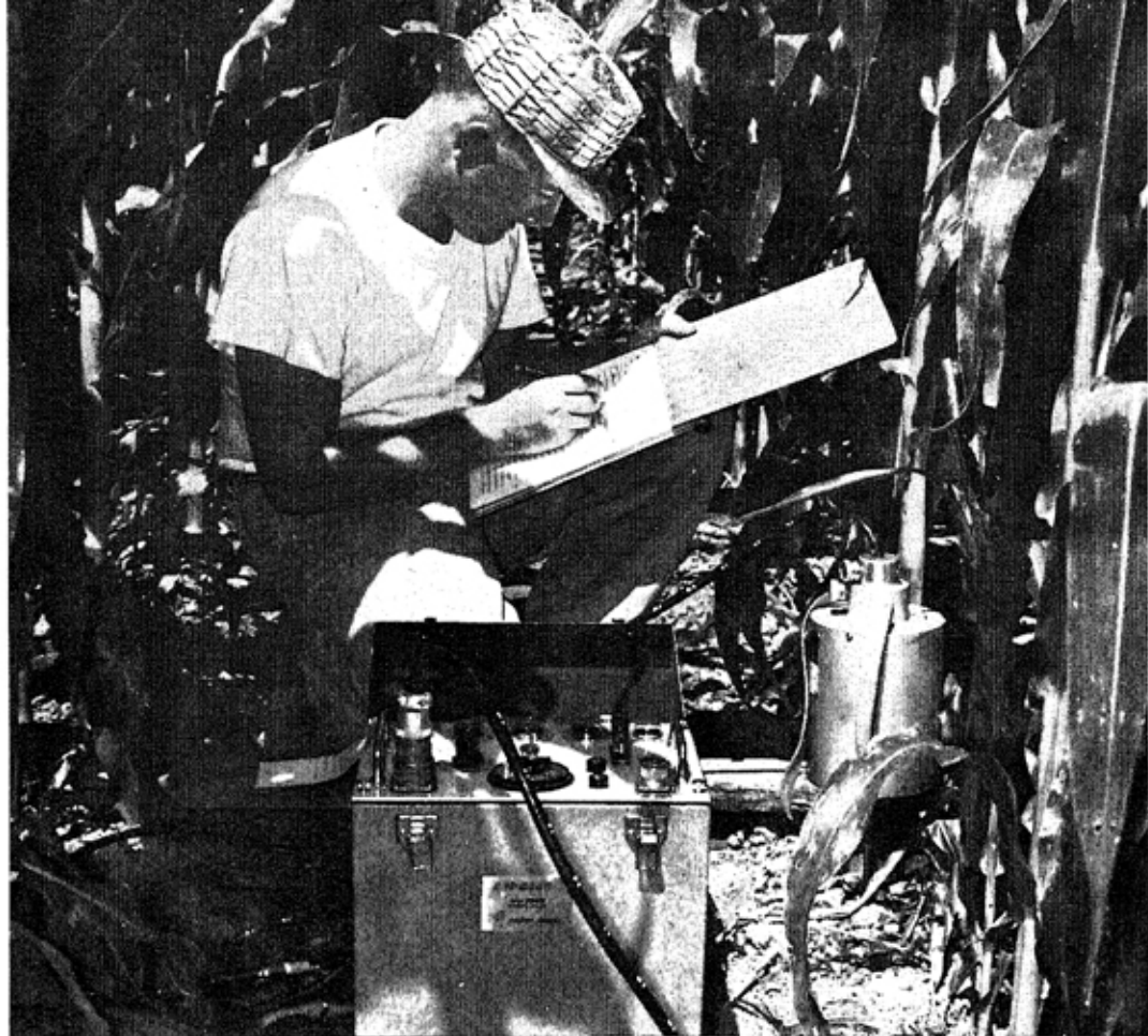
Fig. 6—The soil moisture measurements were taken under the corn by use of the neutron probe on the right and the scalar in the foreground.
