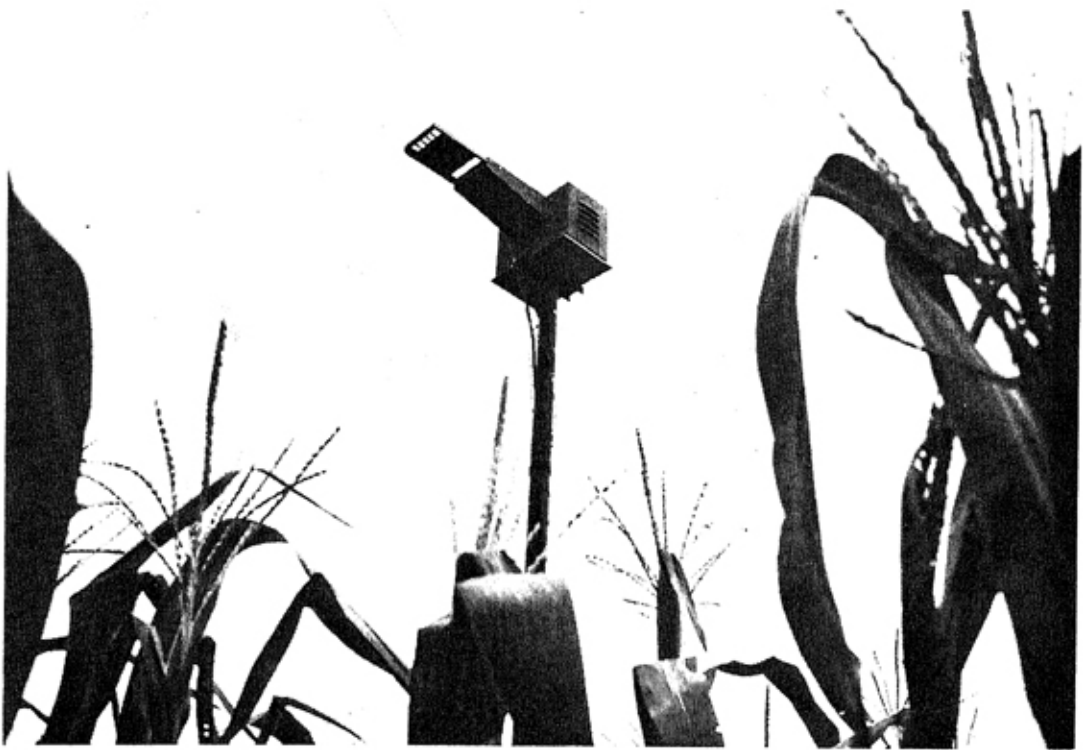
Fig. 1—An instrument used in this study to measure the net radiation above the experimental area used.
