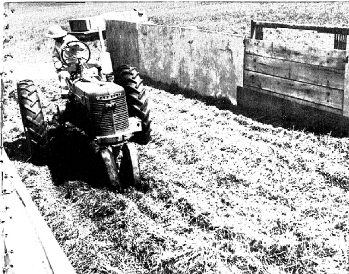
Fig. 2—Roll roofing was used to cover the inside surface of the test panel to prevent silage from wedging into spaces around each plank.
