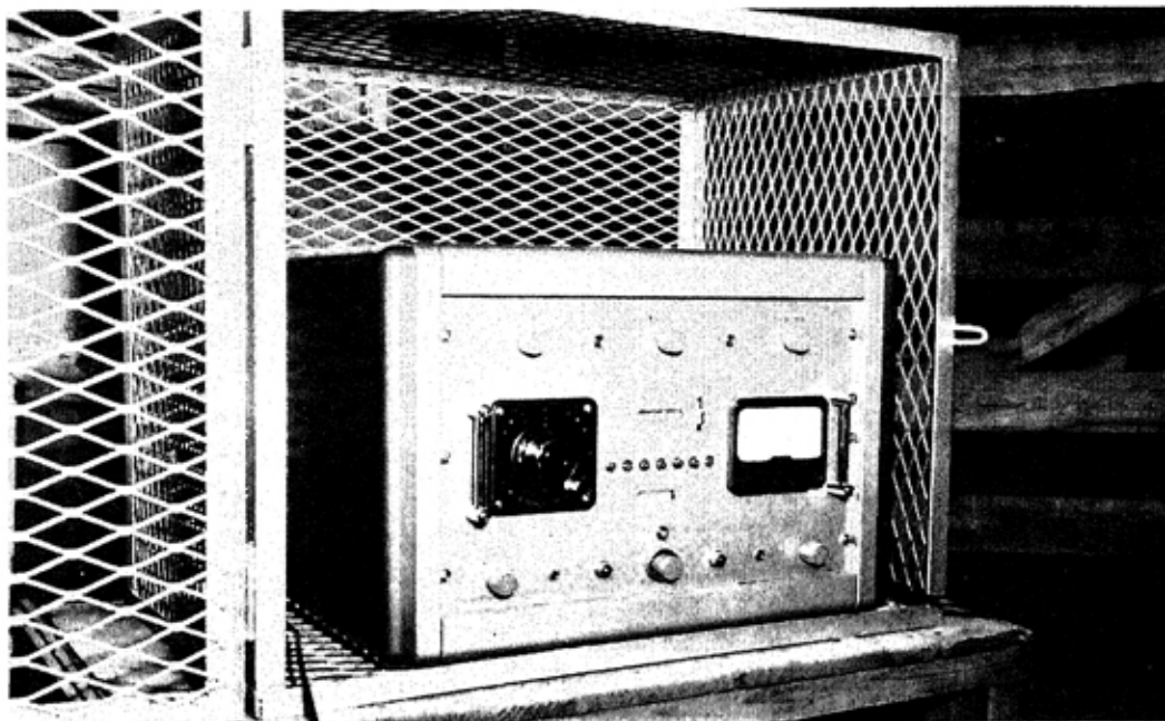
Figure 19—Combination analytical rate meter and scaler unit—employed for measurement of thyroidal I^{131} .
