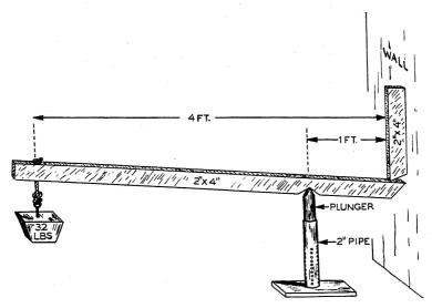
A simple home-made device for determining the moisture content of crops to be ensiled for grass silage.
