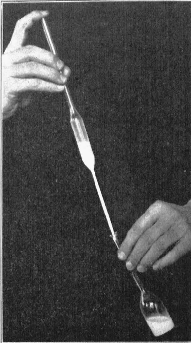
Fig. 4.—Correct way to transfer the milk from the pipette to the test bottle.
