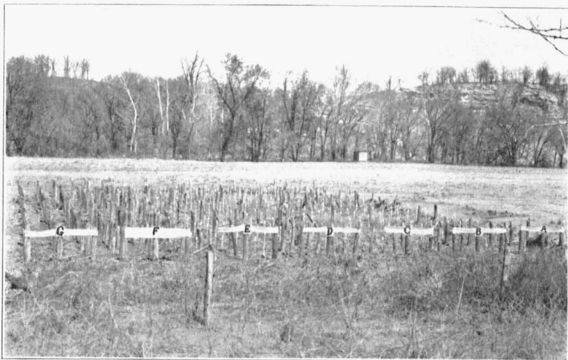
Fig. 2.—Arrangement of posts in seven series to determine serviceable life of each twenty-seven varieties of wood.
