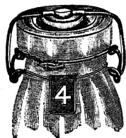
Figure 2. — Milk bottles with metal caps furnish good, air-tight sample jars.
