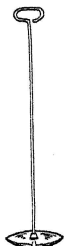
Figure 1.— This stirrer should be used to thor- oughly mix the cream before sam- pling.
