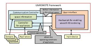
Figure 3: Structure of UbiREMOTE framework
