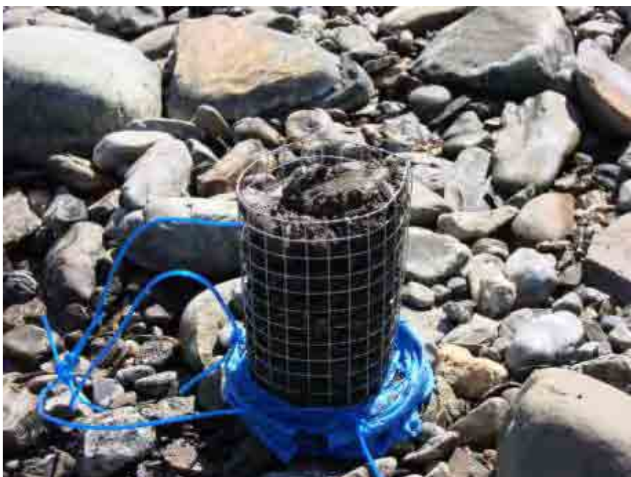
Figure 11: colonisation pot design of 2008, including folded tarpaulin bag with wire-reinforced rim
