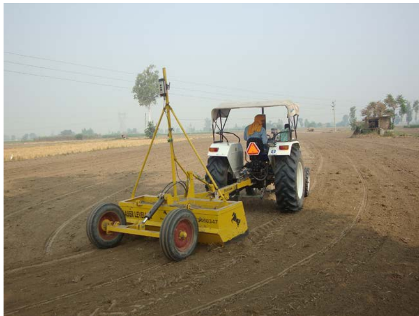
Figure 1. Laser guided precision leveling activity of field in India
