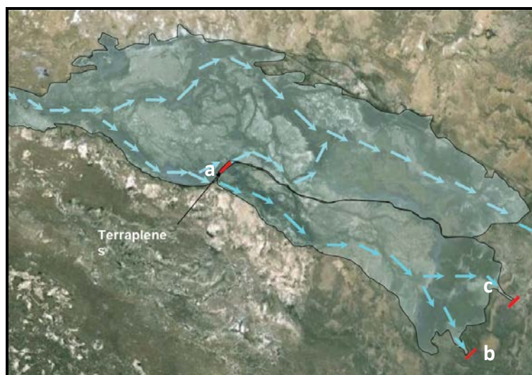
General Works Strategy a) Closure over river arm, b) La Pasarela and c) La Puertita
