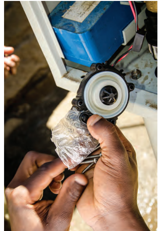
FIGURE 16: COLLINS OUMA, A SELF-TAUGHT METER REPAIRMAN IN NAKURU, KENYA, REPAIRS A LEAKING SEAL WITH A MAKESHIFT PLASTIC GASKET
