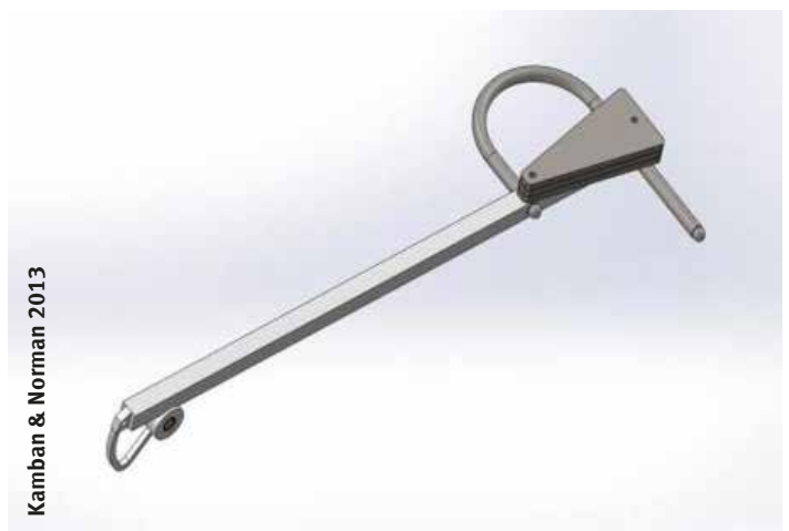
Figure 13: Design of adapted ‘p’ pump handle. User sits on ‘U shape’ side
