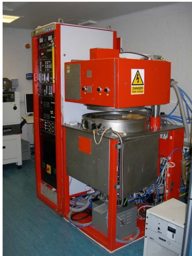
Fig.2- 11 DC and RF magnetron sputtering equipment at Birmingham
