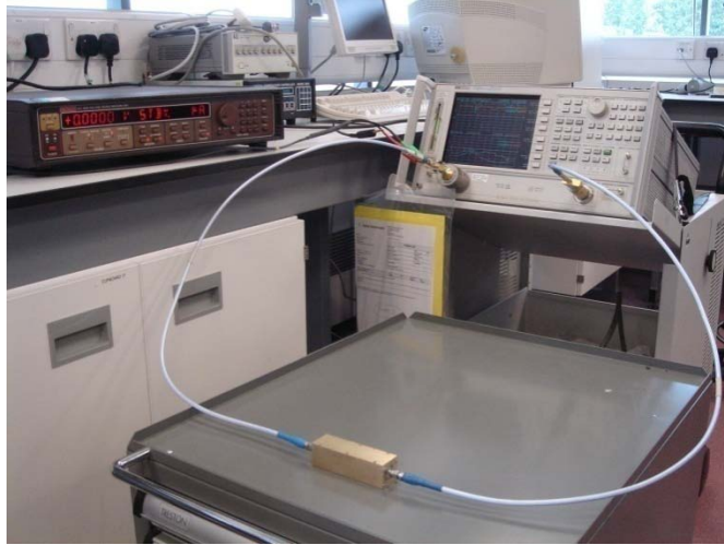
Fig.6- 20 Measurement set-up of bandpass filters in box
