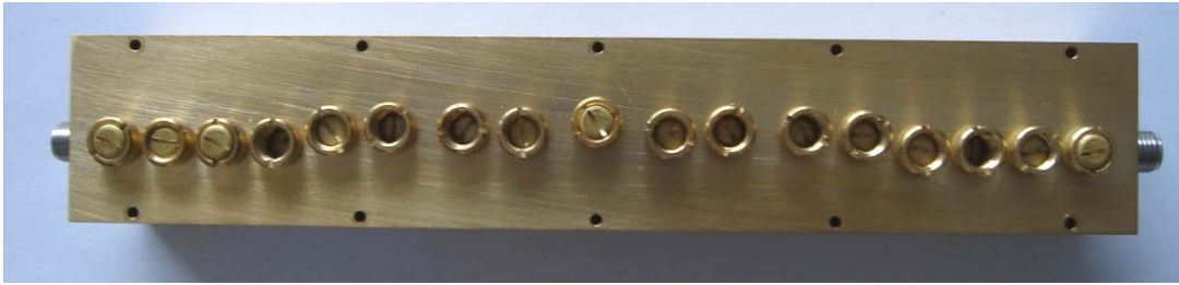
Fig.6- 35 A box with tuning screws for the four pole filter
