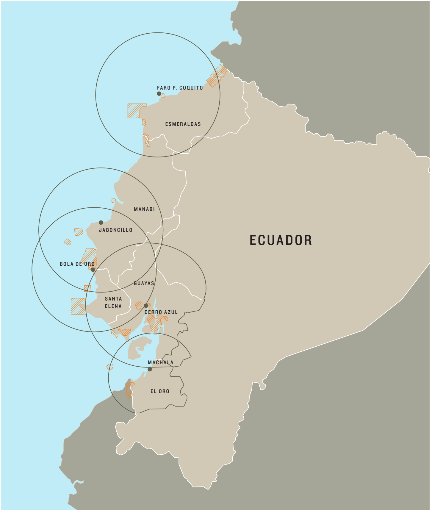
Figure No. 09: Coverage of the VHF Network.
