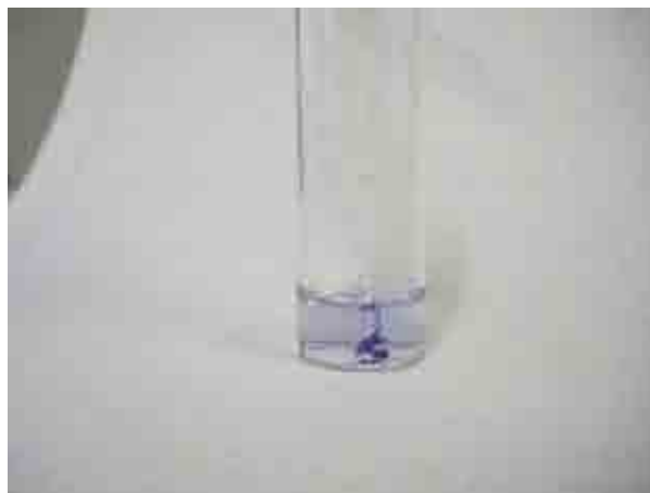
Figure 4.2. 300 \mu\text{M} of ct-DNA with arginine conjugated cylinder. DNA:complex ratio is 20:1 but precipitation of blue strands is visible already at 60:1 ratio.
