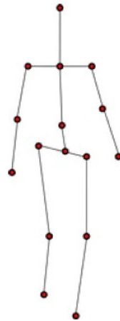
Figure 3.1: Bodies in mass-aggregate engines are represented by a set of particles (red circles) connected by links. The figure shows a character simulation in Twig engine (reprinted without permission from [Horswill, 2008]).
