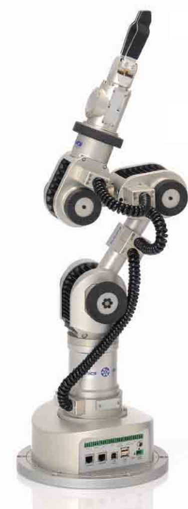
Figure 4.1: The Katana 6M180 robotic manipulator is a 5-DOF manipulator consisting of 5 joints ([Neuronics AG, 2004]). The Katana manipulator also has a gripper with two fingers mounted at the end-effector.
