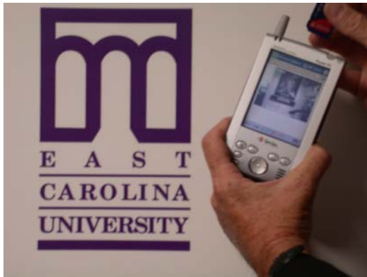
Figure 7: Convergence device consisting of Sprint PCS 3G Smart Phone, Toshiba 2032 PDA, with SD card slot and access to 802.11b WiFi. Photo courtesy of Matthew R. Powell
