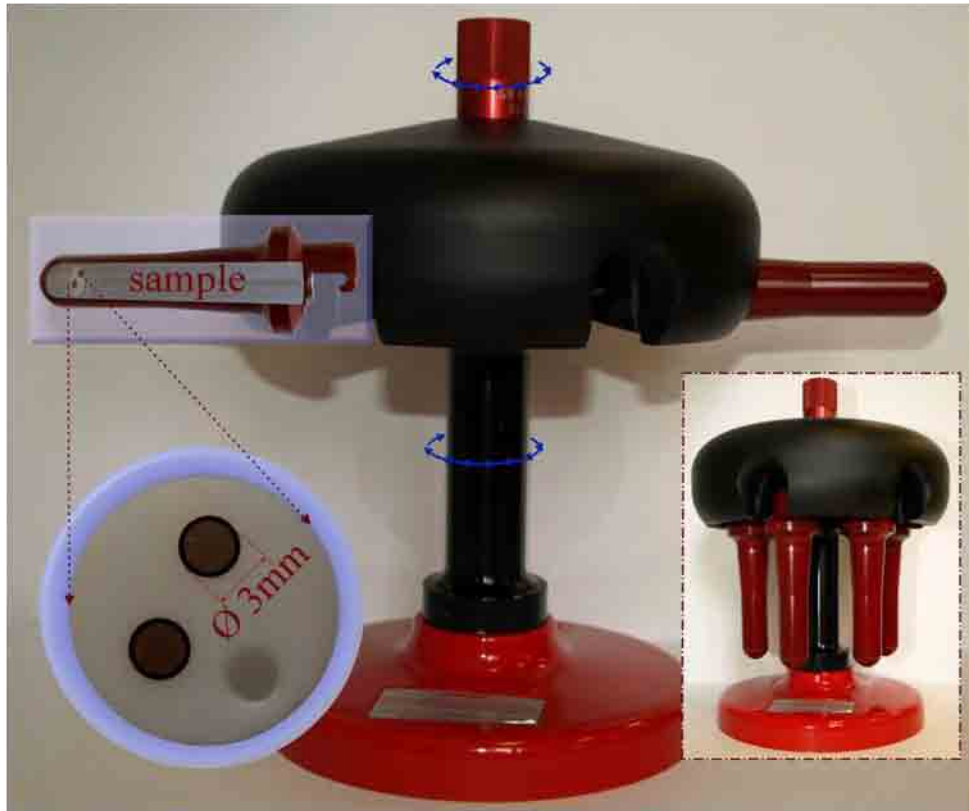
Figure 6.1. Beckman SW40 swinging bucket rotor with a centrifugation tube and TEM grids.
