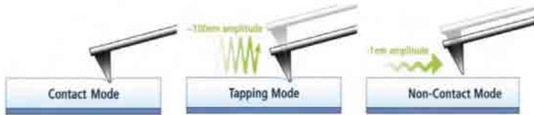
Figure 3.5. Different tip scanning modes of AFM (adapted from Park Systems).
