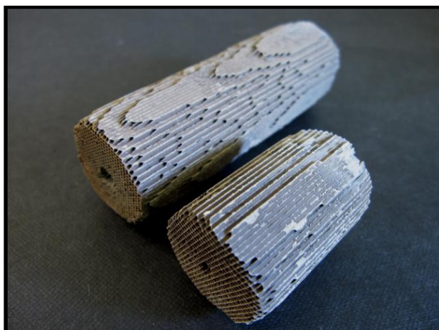
Figure 3.7: Typical monolith fuel reforming catalysts after coring and sizing. The diameter of the catalysts shown here is ~25.4mm.
