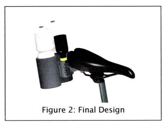
As seen in Figure 2, the setup mounts behind the bike seat with the CO<sub>2</sub> bottle positioned upside down in order to draw liquid and not gas. It is crucial for the design to draw liquid in order to cool more effectively. The preliminary designs used copper coils to run the CO<sub>2</sub> from the tank to the drink holders; by using cast aluminum and an aluminum sleeve we were able to eliminate the need to for tubing. This can be seen below in Figure 3.
