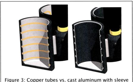
Figure 3: Copper tubes vs. cast aluminum with sleeve
