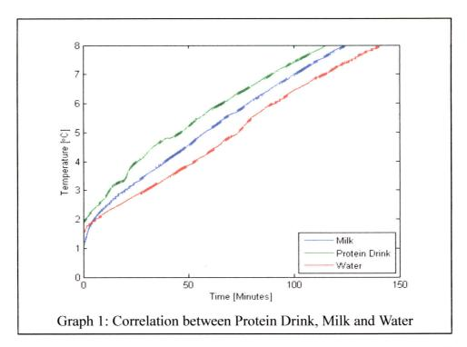
The slopes seem to behave in the same manner, but to make sure a linear fit was applied through a built in function in MATLAB, which can be seen in Appendix [2]. The values of the slopes all hover around 0.05°C/min, which can be seen in Table 1.
