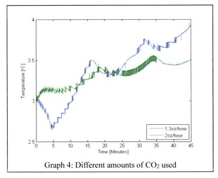
A linear fit was applied to this new graph and was found to be 0.01°C/min. That is half of what the 1.3oz/hour had. Extrapolating this, it would now take 420 minutes for the protein drink to reach 7.2°C, or 7 hours. The CO<sub>2</sub> however, would run out in 6 hours. By releasing 2oz of CO<sub>2</sub> per hour, the total time on the bike was increased to just above 6 hours.
