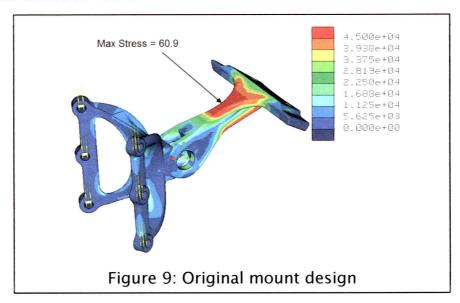
Several iterations were conducted to get the stress in the one area as low as possible. The necked down area of the link was made significantly thicker and the location around the bolt holes were made bigger to allow the stress to flow from the bolt holes to the thinner section of the link. The final iteration is shown in Figure 10. It has a maximum stress in the neck of the link of 22.9 MPa.
