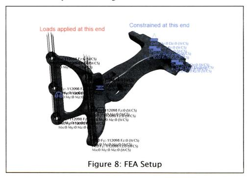
The area that needed to be analyzed more closely was the link from the bike saddle mounts to the solenoid valve. The analysis was done on these two components only to speed up the iterations. The original setup/design is shown in Figure 9. The max stress in the necked down area of the link was at 60.9 MPa.
