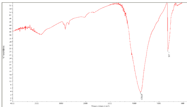
Figure 9. FTIR spectra obtained for GR-04 after purification. Usual BNNT peaks were observed.
