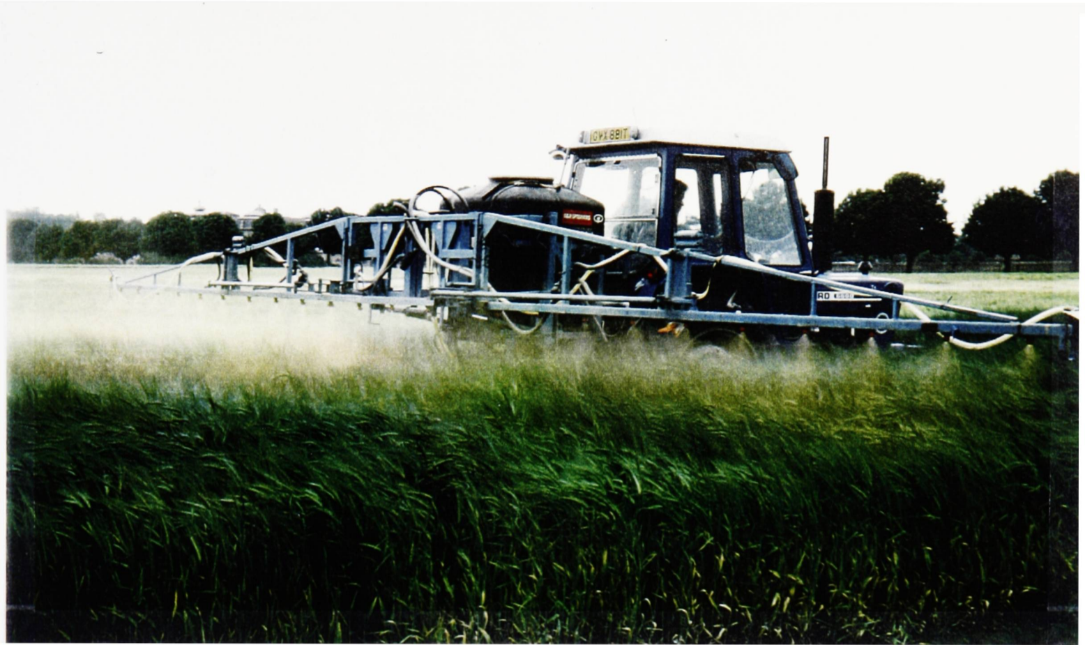
1. A typical agricultural boom sprayer during operation. The 18 m boom of overlapping sprays (geometry as in figure 2 below) is mounted 0.5 m above the plant canopy top. The vehicle is moving at 6 mph into a light breeze ( 1.5 \text{ m s}^{-1} at boom height). Note the region of airborne spray behind the vehicle (photograph courtesy of Silsoe Research Institute).
