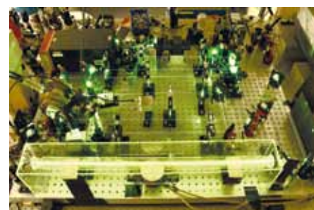
FIG. 3: Photograph of the iodine standard at the Humboldt-University Berlin utilizing an 80 cm long iodine cell (shown in the front).
