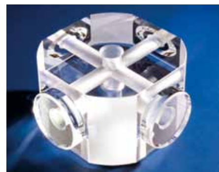
FIG. 5: Photograph of the high-finesse cavities used at the Humboldt-University Berlin for a Michelson-Morley experiment.
