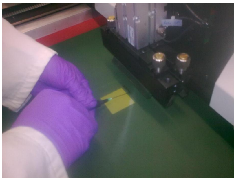
Figure 55 - Image of painting method for fabrication of GDEs.
