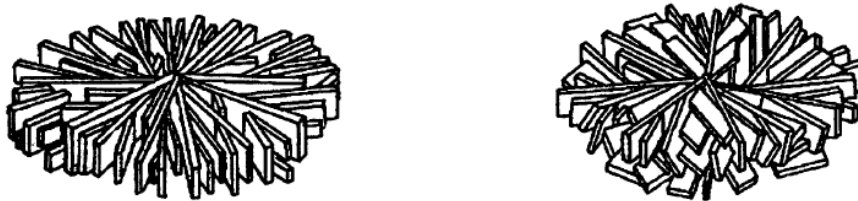
Figure 1.8 Schematic representation of a highly oriented, edge-on PEEK spherulite (left) compared to that of a typical polymer (from Lovinger and Davis, 1985).
