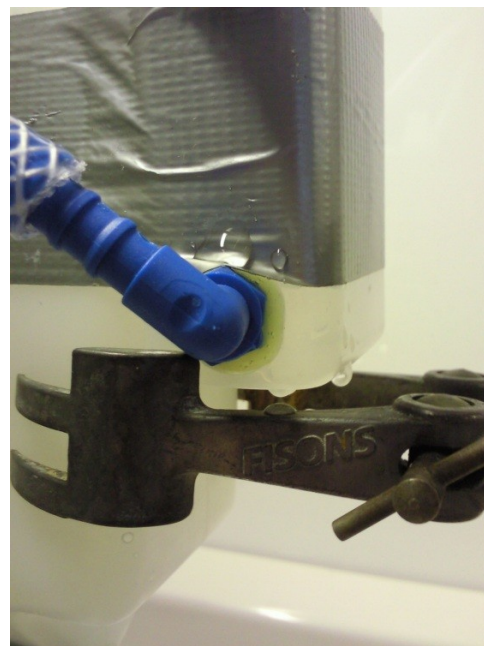
Figure 23: Image showing small leak on side tank
