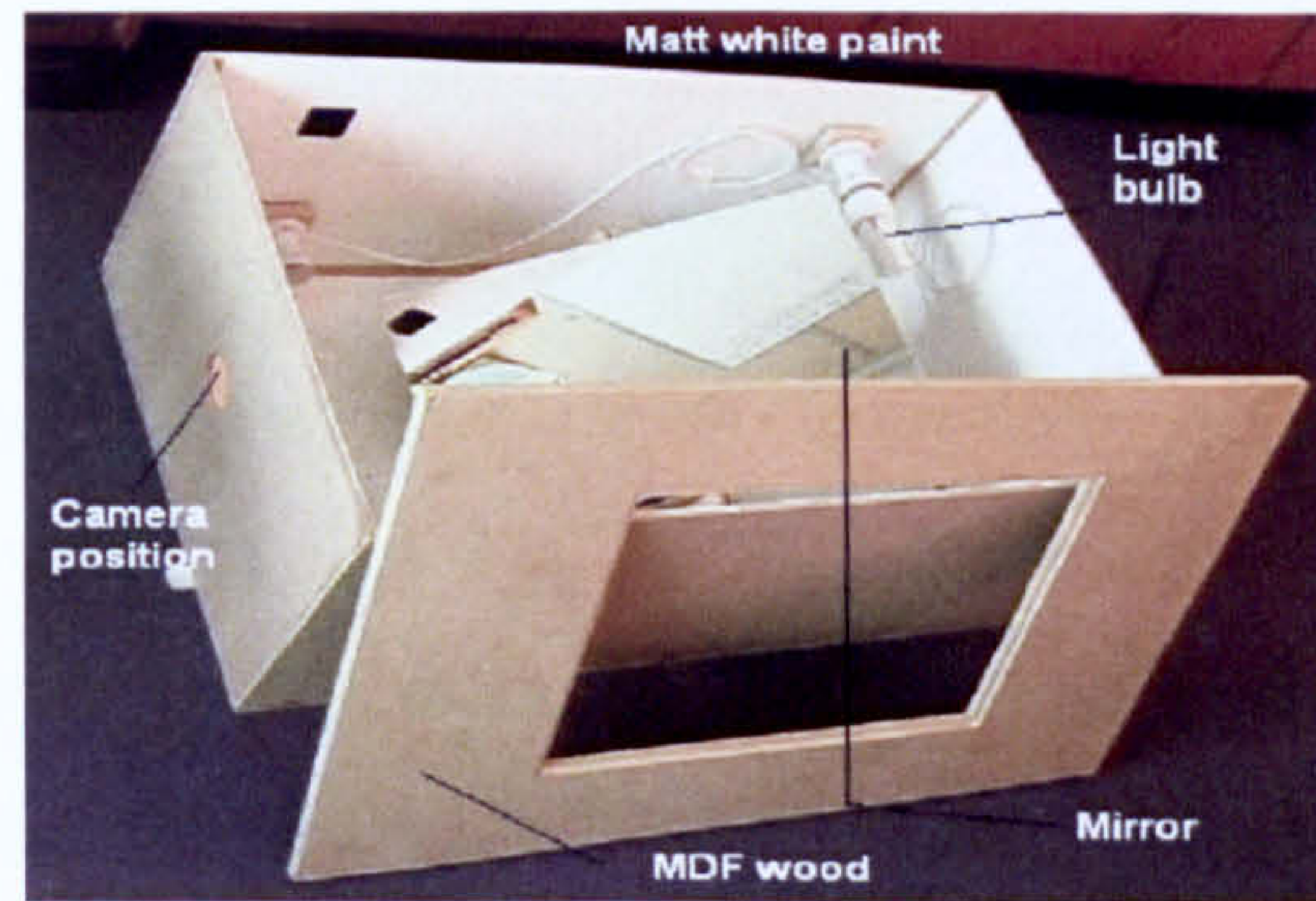
Photograph 4-1: Photograph of the first prototype measurement platform.
