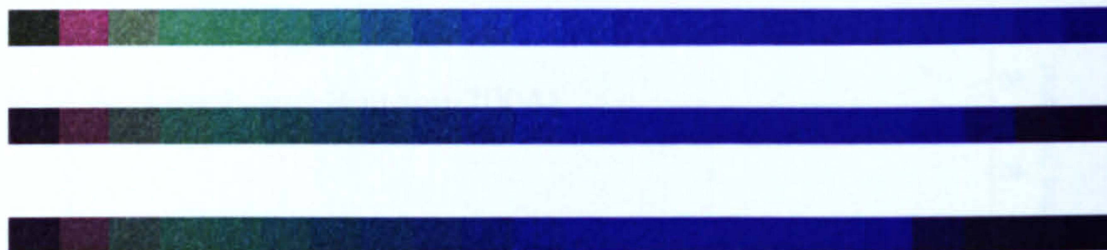
Figure 5-16: Calibration bars for the heating and cooling runs. Notice the reduction in intensity of colours throughout the colour play interval for the cooling runs.
