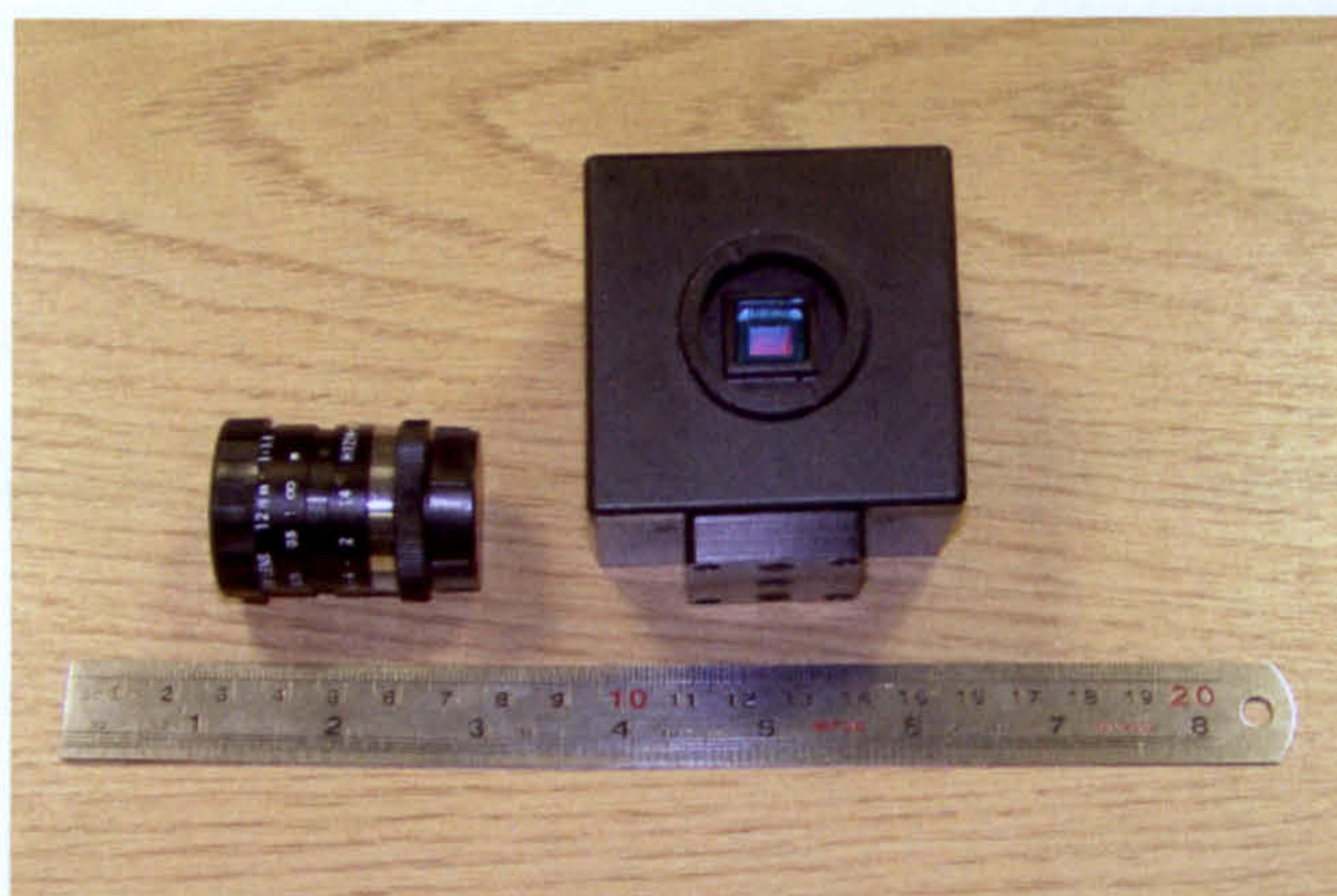
Photograph C-1: Single CCD RGB camera based on IEEE 1394 protocol and its associated mount lens.
