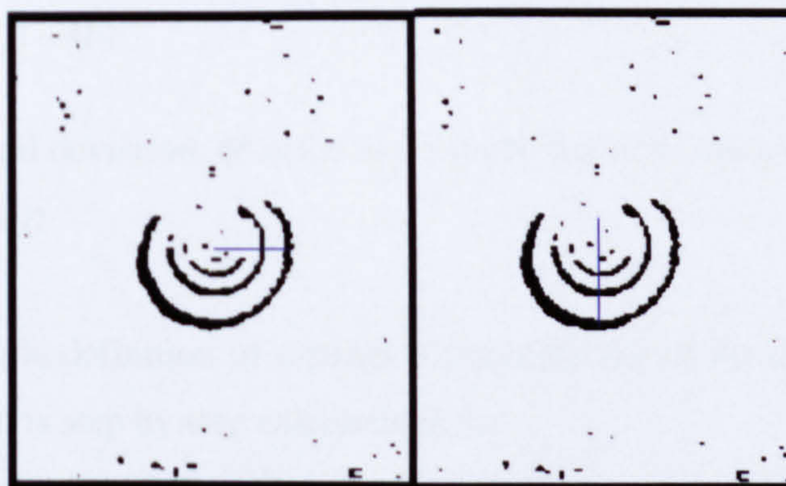
Figure 9: Segmented images with measured vertical and horizontal span
