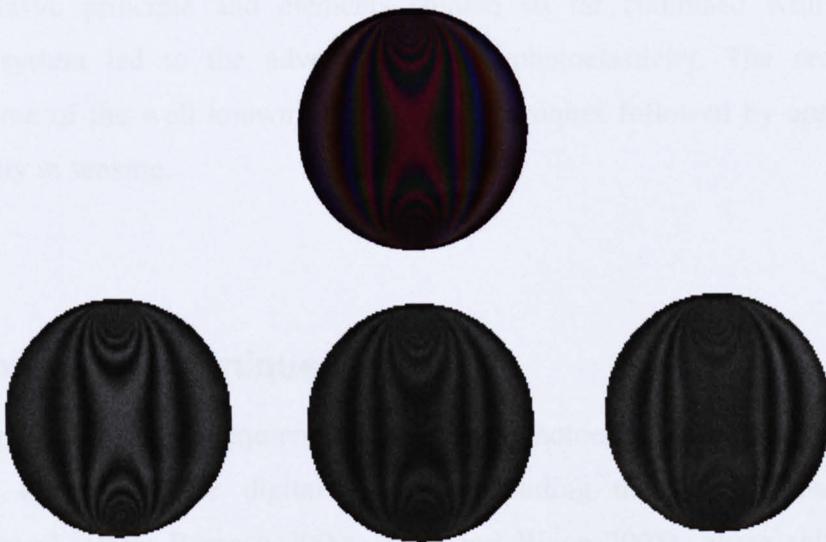
Figure 2-8: An RGB photoelastic image with isolated R, G and B planes for individual image plane comparison in terms of spectral response
