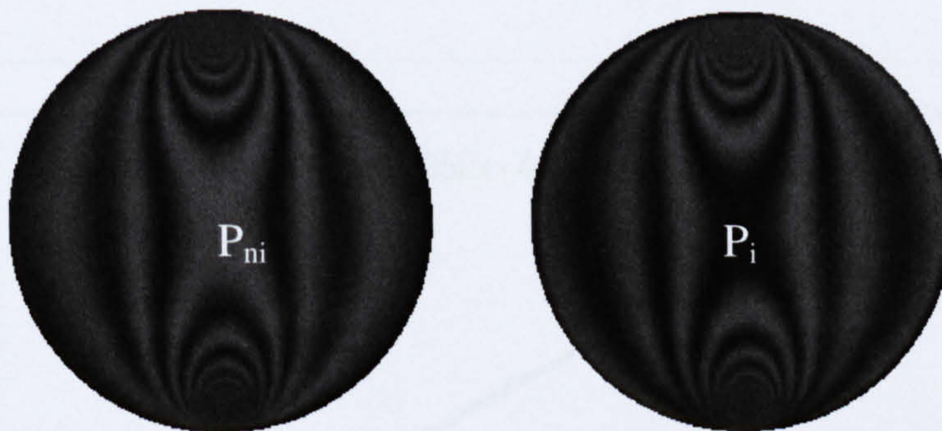
Figure 3-8: Tardy's compensation (a) non-integral fringe order at 'P ni ' (b) integral fringe order at 'P i ' after rotation of polariscope (circular polariscope configuration)
