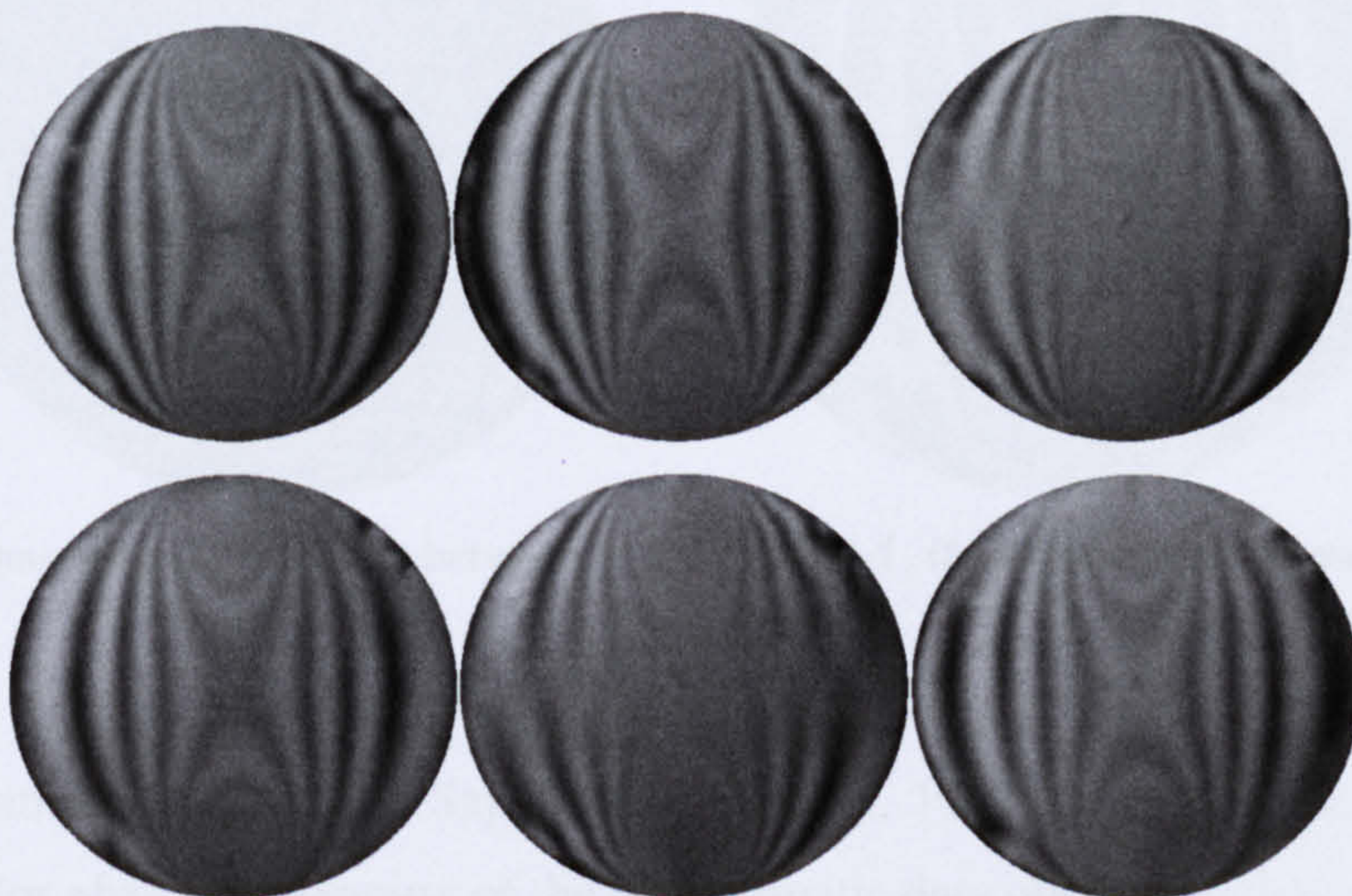
Figure 2-9: Six phase stepped images for phase-shifting technique acquired in reflection mode for a disc under diametral compression
