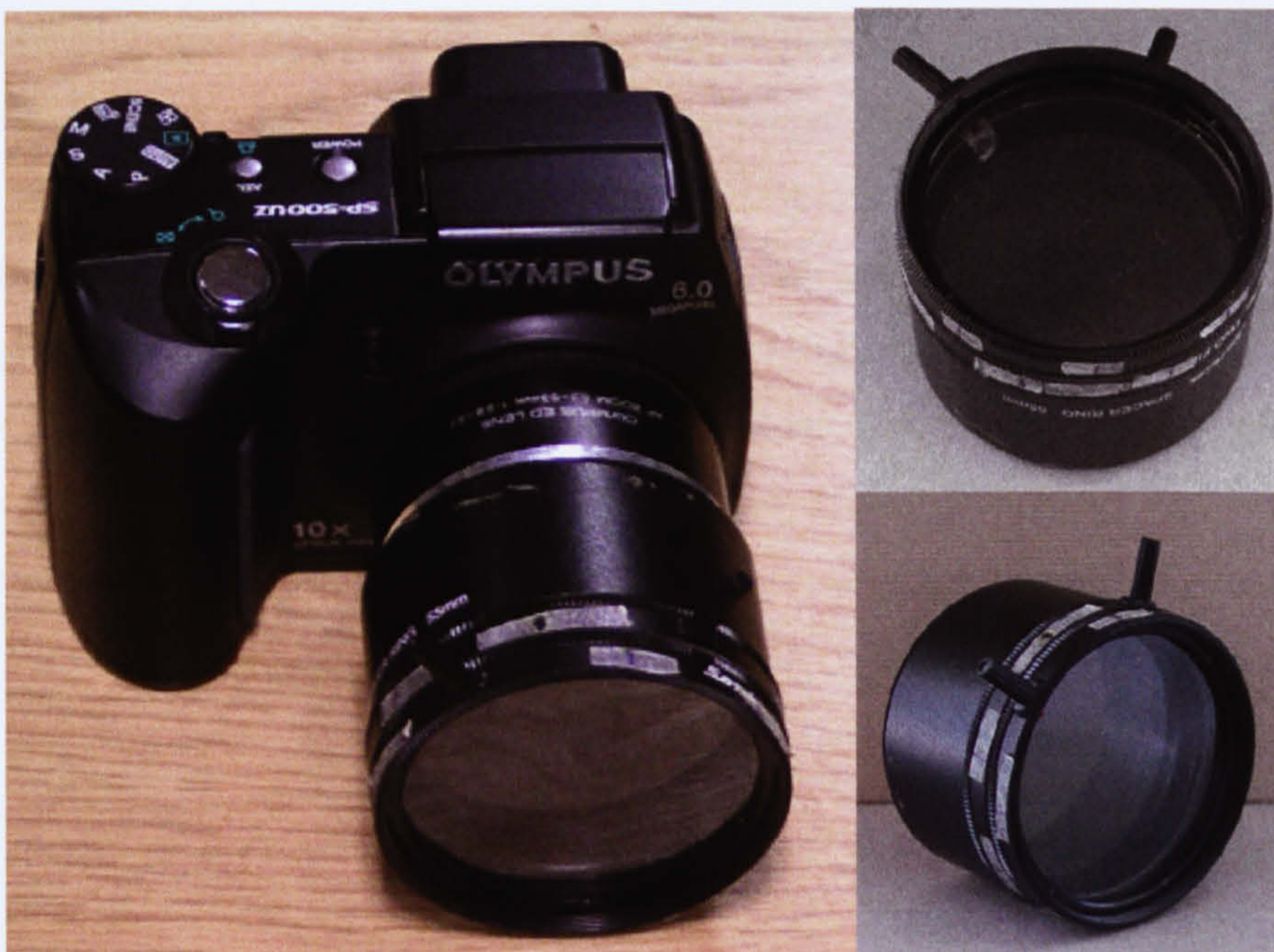
Figure 3-18: (a) Digital Camera used in the experimentation, (b) optical mountings with independent rotation of polariser and quarter wave plate
