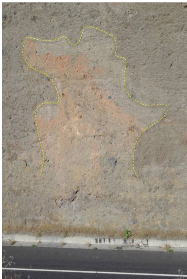
Figure 7 – Flame injection structure at a roadcut within the Popocatepetl VDA deposit. Texture of the flame structure is finer grained as compared to the coarse material above and adjacent. Scale of structure approximately 10 m.
