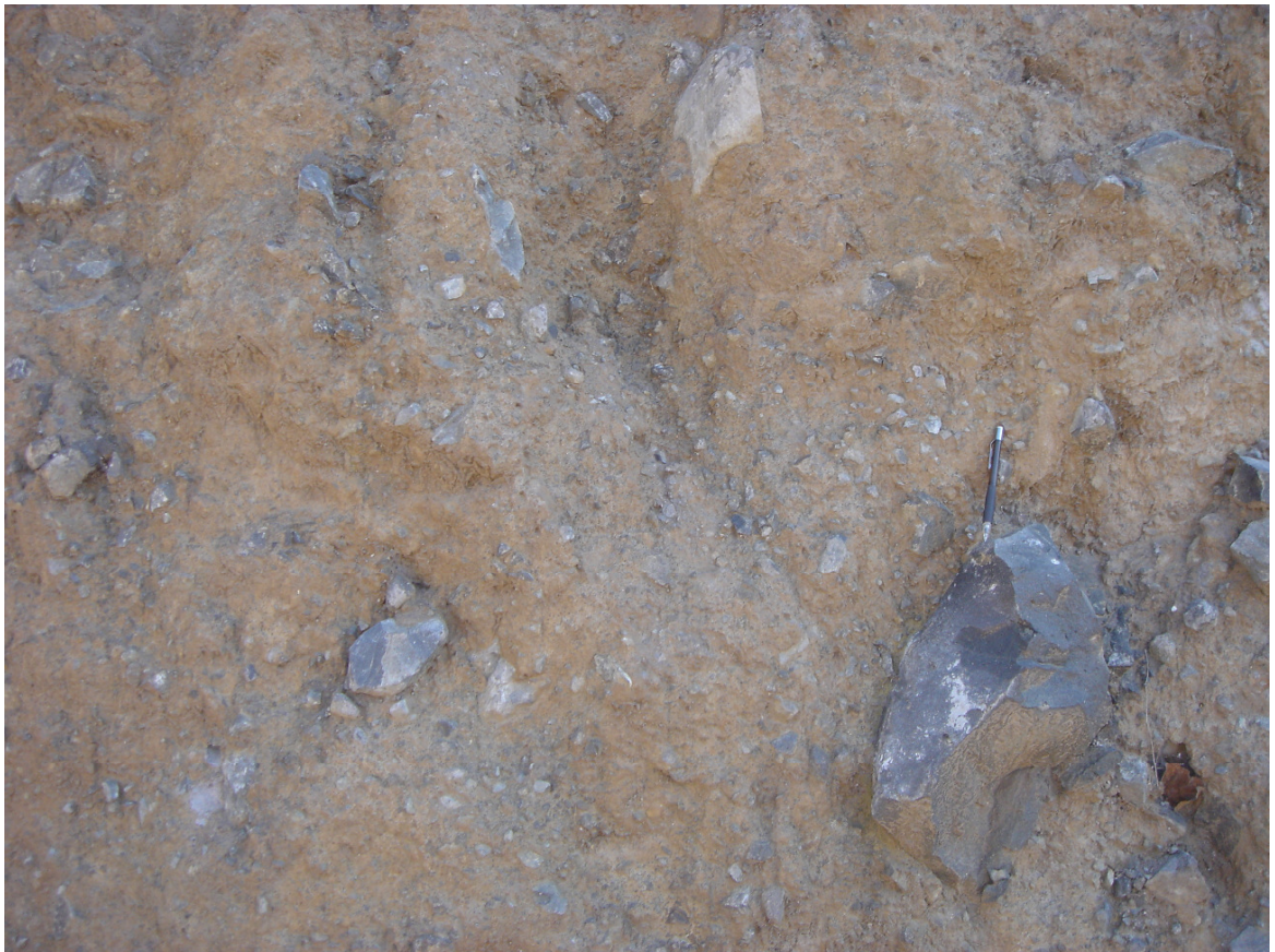
Figure 3 – Matrix material of the Popocatepetl VDA deposit displaying a generally fine-grained texture with chaotic assortment of angular blocks of various sizes. Pencil for scale (14 cm in length).
