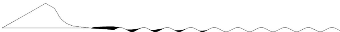
Figure 81 – Sinusoidal runout space pattern showing both a pre- and post-failure scenario where the failure material piled up into the proximal topographic basins. In this case wave patterns have a wavelength, \lambda , of 940 m and an amplitude, A , of 170 m. Full cone height is 1,000 m.
