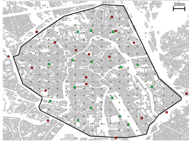
Figure 5.4: The selected suburban area of 6.85 \text{ km}^2 in Ghent, Belgium. Users are located on the yellow dots; squares indicate base station (BS) sites. As an illustration of the sleep mode principle, the active and inactive BSs for a simulation with 70% available power and random user distribution are colored green and red, respectively.
