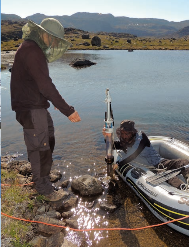
Bringing a core (taken using a so-called UWITEC corer) from the bottom sediment of a lake in the Kapisillit area to shore (Dagmar Obbels).
