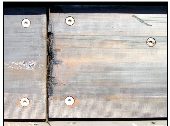
Fig. 8. Jute fibre/phenolic resin composite slipway lining wear: Longitudinal panel edge wear
