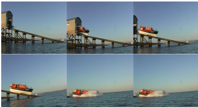
Fig. 1. Typical slipway launch: Tyne class lifeboat at Selsey moves down the plain sliding section of the slipway under its own weight
