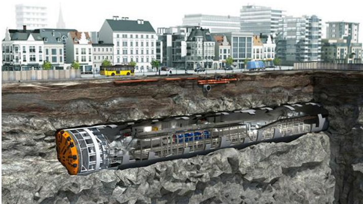
Figure 4.3. Illustration of a tunnel boring machine working under a city (ixtract GmbH, 2014).
