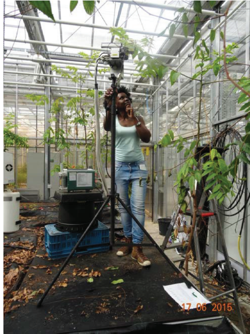
Figure 3.1 Photosynthetic measurements being done on an M. eminii seedling using a LICOR in the tropical greenhouse at ILVO
