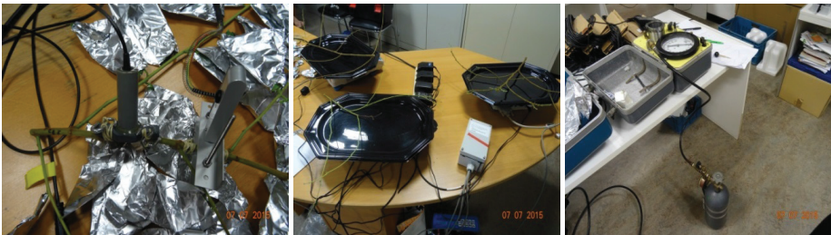
Figure 4.3 Left to right: An excise M. eminii branch with leaves wrapped with foil (set 1) and onto which an acoustic and dendrometer have been attached. The branches stripped of their leaves (set 2) can be seen placed on black plastic plates. The pressure bomb used in xylem water potential measurements.
