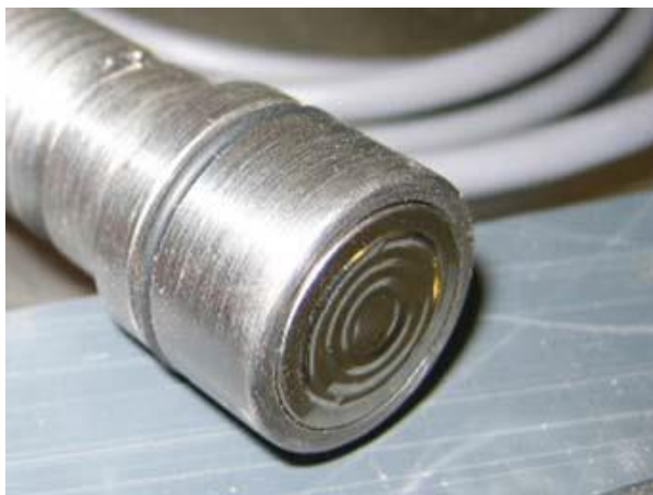
Fig. 5-11: Electronic pressure sensor type 2 [5.7].
