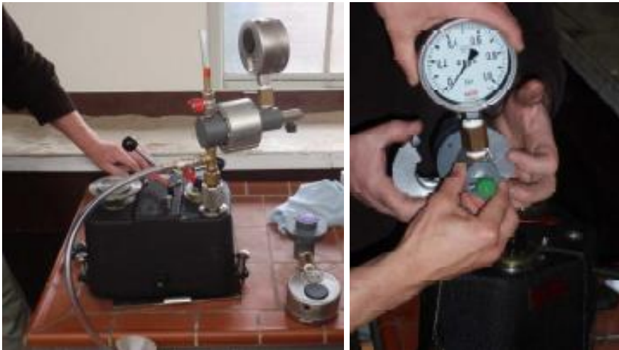
Fig. 5-2: Pressure measurement system.
