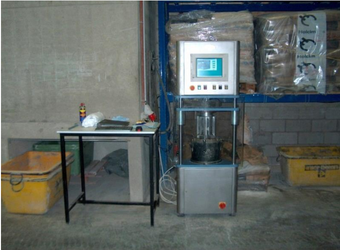
Fig. 2-14: General layout of the BML Contec-Viscometer 5.
