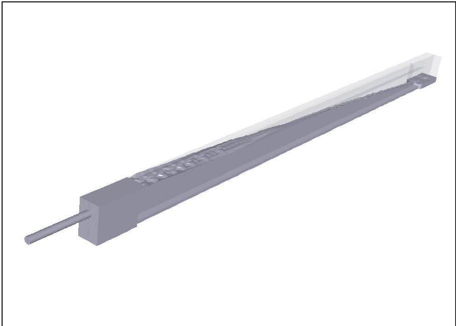
Fig. 6-32: Simulated filling process of the I-beam.
