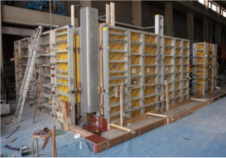
Fig. 5-1: Layout of the four formwork base-filling tests.
