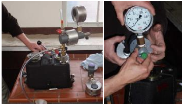
Fig. B-4: In-house developed pressure measurement system.
