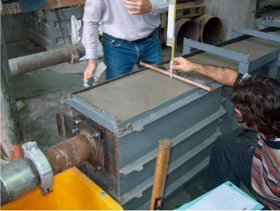
Fig. 6-33: SCC surface just after the inlet at the end of the I-beam filling process.
