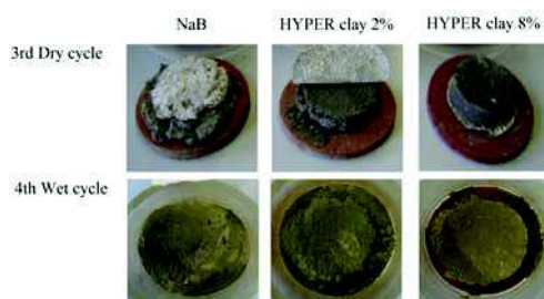
Figure 2. Specimens at the end of the third dry cycle and at the end of the fourth wet cycle
