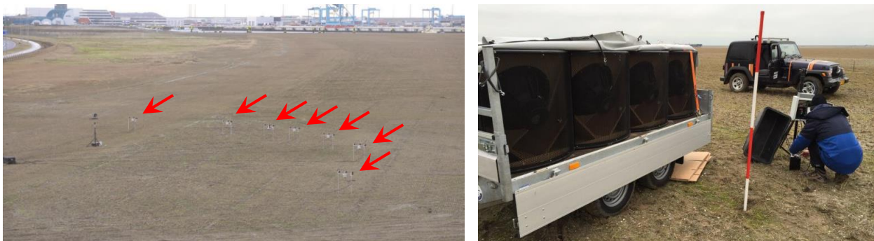
Figure 4: Photographs of the microphone array setup (left, subarrays are indicated with an arrow) and of one of the trailer-mounted test loudspeaker systems used for the field test (right).
