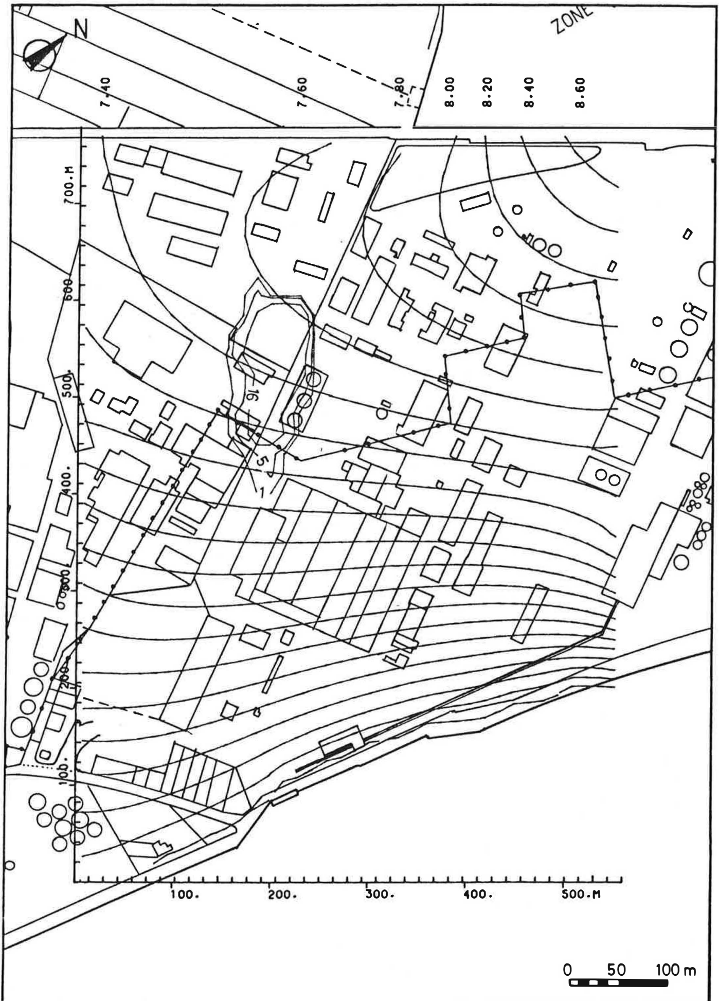
Fig. 28 - Simulation H1 - situation after 15 years (1987) (one spill area during 1972 - 1979,5 only normal infiltration during 1979,5 - 1987)
