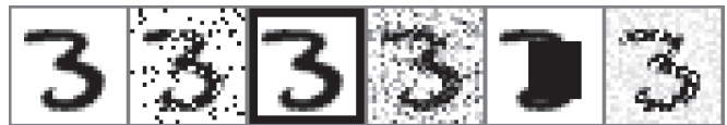
Fig. 1. From left to right, a clean MNIST sample and its corresponding noisy versions: salt & pepper, border, Gaussian, block, and speckle, respectively.
