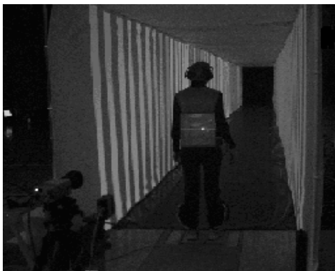
Figure 1: Subject ready to start in the hallway for control condition C (non-moving stripes). The reflecting cardboard was used to receive accurate data from the distance laser.
