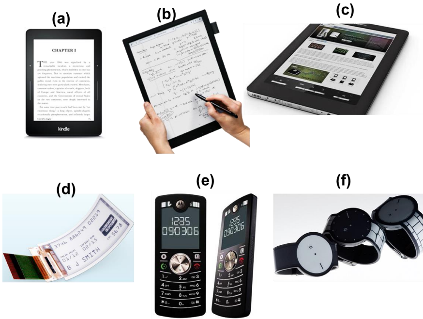
Figure 1.2: A few devices based on V-EPDs are shown. In (a) the Amazon Kindle ebook reader is an example of a typical monochrome reflective display featuring low power consumption (b) the Sony E-ink based tablet: Sony DPTS1 digital paper system (c) E ink's triton color EPD offers 16 levels of gray scale and is able to displays 4096 colors – be it in a poor color quality (d) Plastic logic e-ink based flexible displays (d) Motorola Motofone (e) Sony's FES e-ink based watches.
