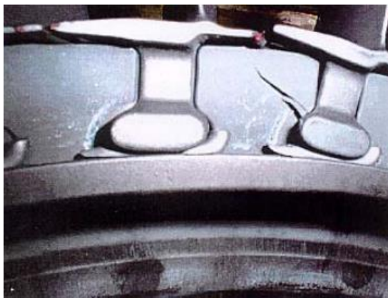
Figure 2-11. Fretting fatigue of the blade and disk connection [43]
