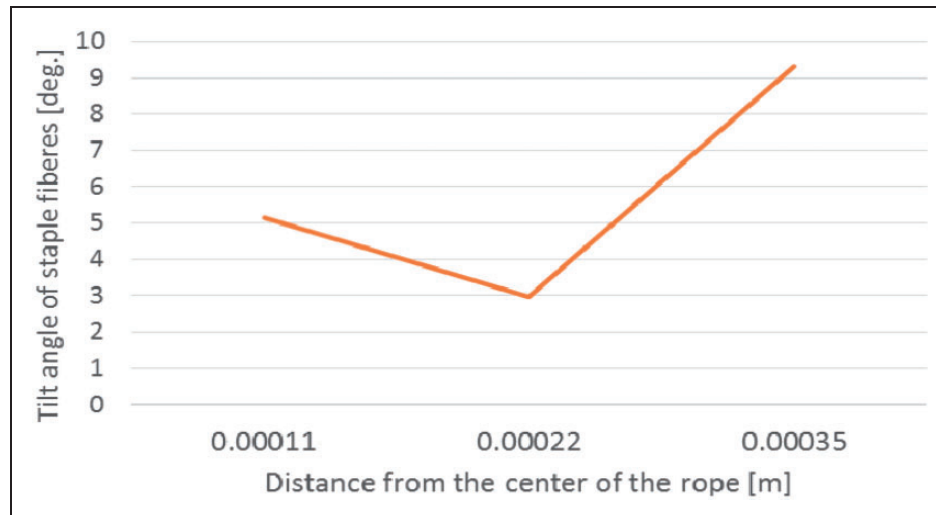
Figure 9. The dependence between the tilt angle of the staple fibers and their distance from the center of the rope.
